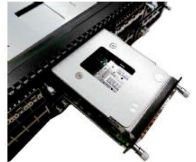
Insert the network module tray back into the bay.
