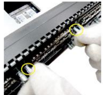
Tighten the captive screws to secure the network module in place.
