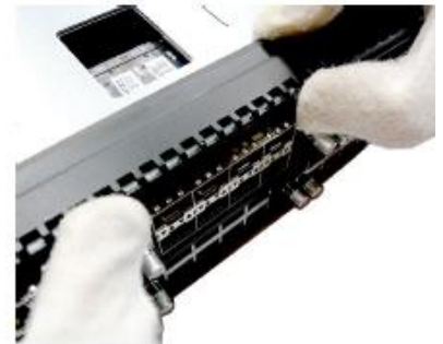
Push in the tray to fully seat the network module.
